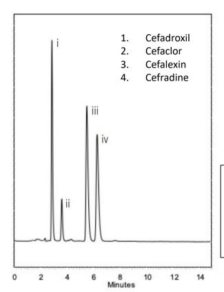
Column: Horizon Phenyl, 5μm 150x4.6mm
